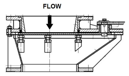
Special care should be taken to maintain the correct distance between the flanges and to ensure that they are parallel to the valve body. Incorrect alignment of the valve can cause deformations, which can lead to difficulties in operation.
